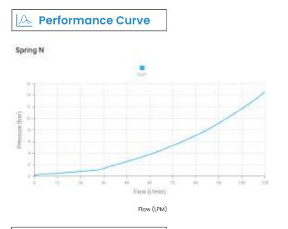
Note: The performance chart illustrates flow handling capacity. p/Q curves are recorded at TOil = 40°C and 46 cSt.
